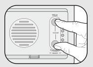
Press and hold both buttons on the intercom for 5 seconds. An initial beep will be heard followed by a second beep. The channel lights will flash. Within 10 seconds put the second intercom into Learn Mode (refer to table below).
